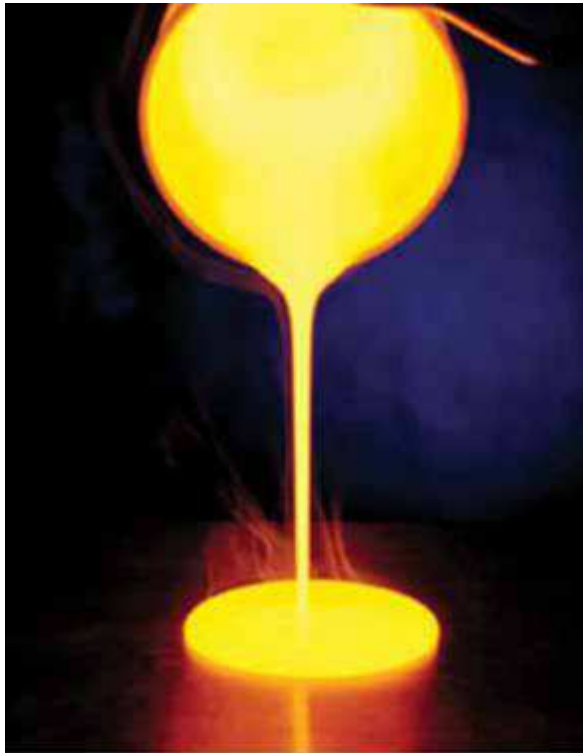
VITRIFICATION Pouring glass to immobilize radioactive waste.
