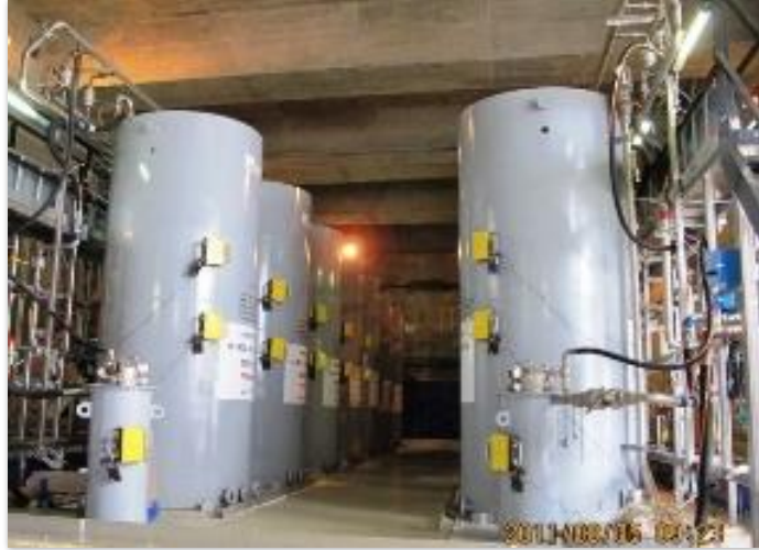
SARRY (Gen-1) Fukushima – 2011 Air Annulus Limited Cs Loading
