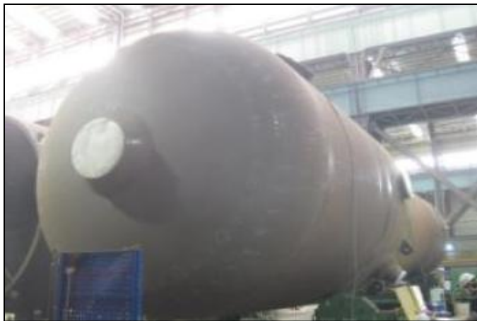
Hydro test Complete for Unit 2A SG
