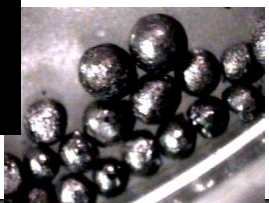
Uranium carbide kernels fabricated at USC using the rotating electrode method
