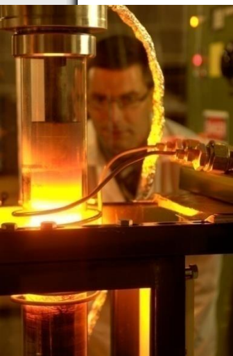
Fluidized-bed CVD Coater built at USC
