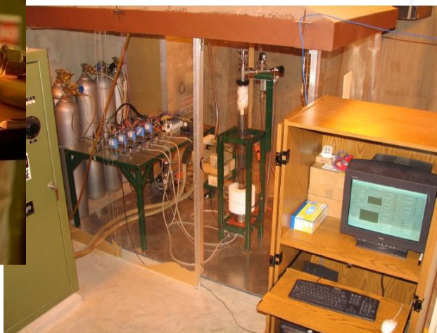
Fluidized-bed CVD Coater built at USC
